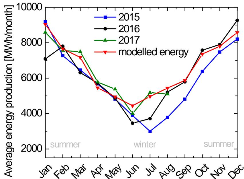
**FIGURE 3.** Modelled and produced monthly energy of the Touwsrivier power plant in the years 2015, 2016, and 2017. The modelled energy was calculated with PVsyst and additionally considers several PV specific loss factors, e.g. soiling and degradation.
