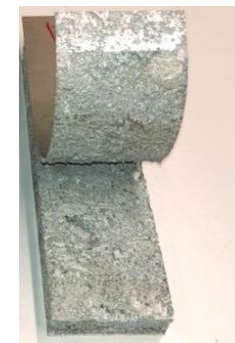
Failure in the core Sandwich VII, Probe 3
