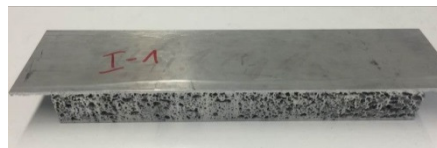
Peeling sample Sandwich I, Probe 1
