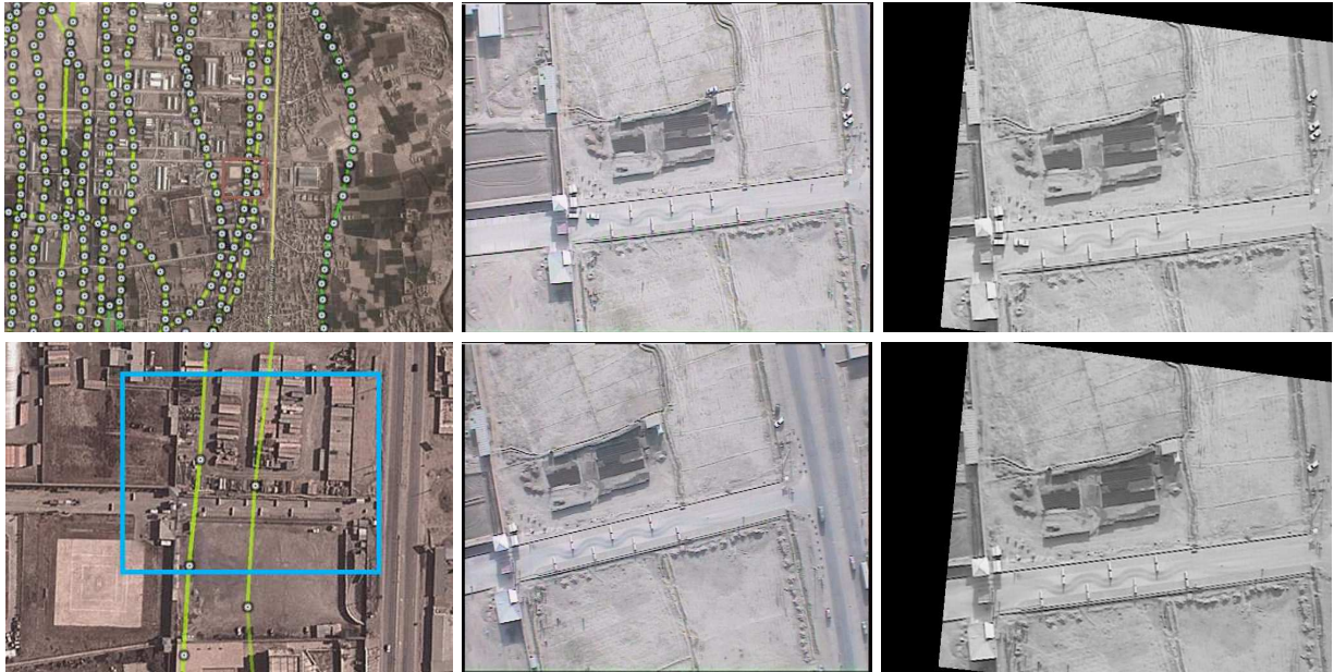
Figure 1. Frame selection for example scene access point from satellite image with overlaid flight path (left column), selected frames from two overflights (center), and registered images with non-overlapping areas masked out (right).
