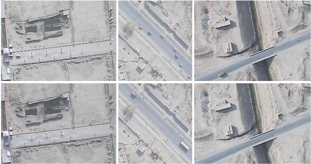
Figure 2. Registered and clipped color image pairs for change detection from example scenes access point in the left column, road in the center column, and bridge in the right column.
