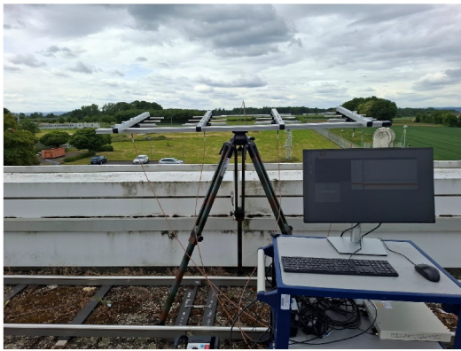
FIGURE 7 | View on the four-element antenna array on the roof of a building at the site of Fraunhofer FKIE.
