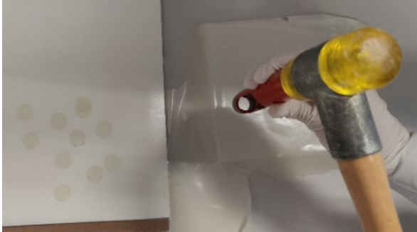
a) Punching out of the epoxy foil
