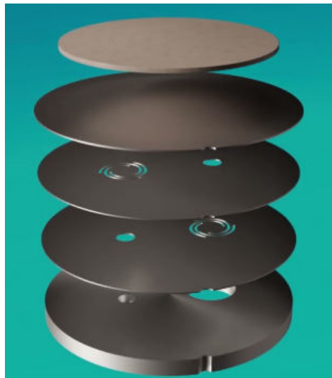
Figure 8 Components of the micro pump base body [50]
