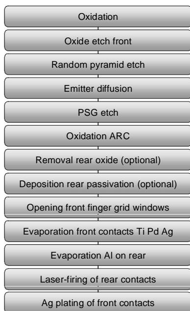
**Figure 1:** Workflow of the manufacturing of the high-efficiency cells presented in this work.
