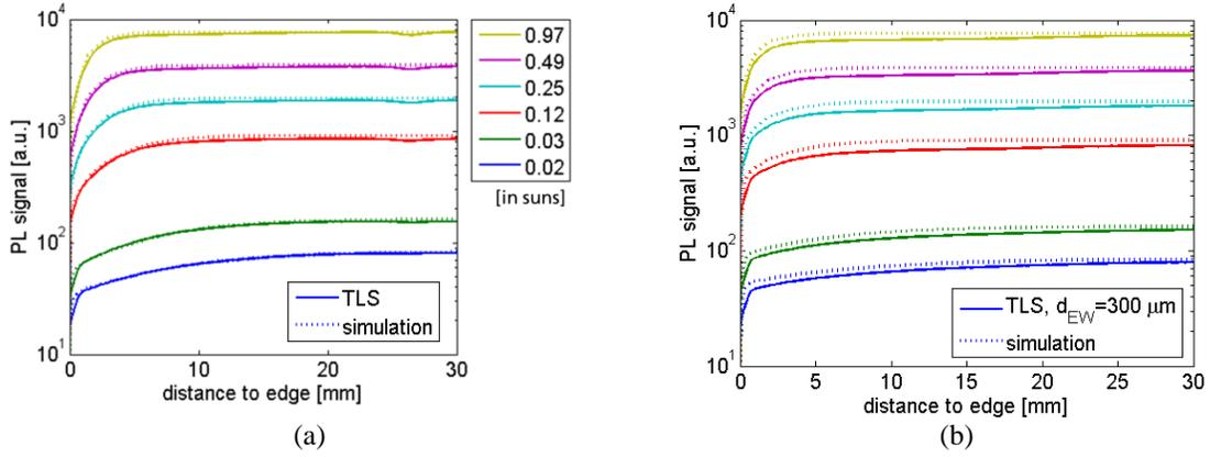
**FIGURE 6.** Comparison of the experimental and simulated data of the TLS edge using the best-fit, which is shown for all six illumination intensities in (a) for the TLS edge with  $J_{02,edge} = 3$  nA/cm and  $S_{eff,edge} = 10^5$  cm/s and in (b) for the TLS edge with emitter window with  $S_{eff,edge} = 10^5$  cm/s.
