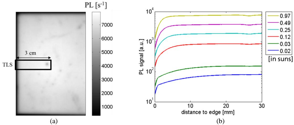
**FIGURE 2.** (a) PL image at 0.97 suns; (b) PL profiles at six different illumination intensities for the TLS separation through the pn-junction.
