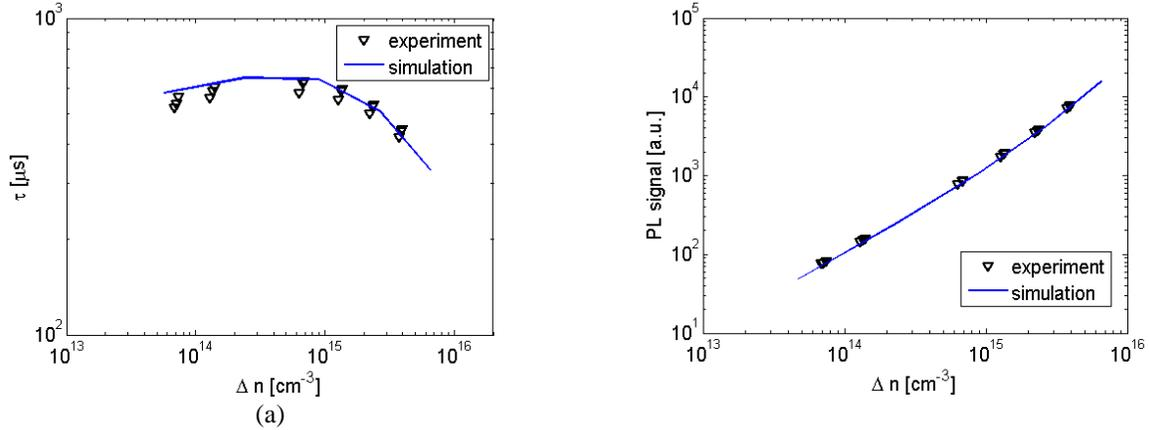
**FIGURE 4.** (a) Excess charge carrier density  $\Delta n$  dependent effective lifetime  $\tau$  curve whereas three homogeneous spots in the middle of the wafer which are not influenced by the edge are chosen. The fit parameters of the simulation are  $J_{0e} = 70 \text{ fA/cm}^2$ , midgap related bulk lifetimes  $\tau_{p0,\text{bulk}} = 1.5 \text{ ms}$  and  $\tau_{n0,\text{bulk}} = 50 \text{ ms}$ ; (b) calibration of the PL intensity.
