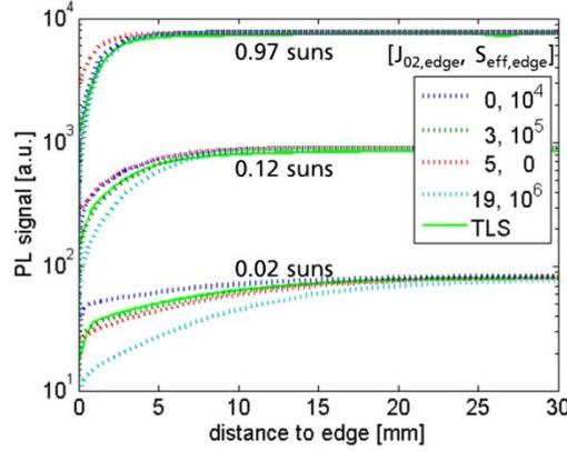
**FIGURE 5.** Comparison of the experimental data of the TLS edge through emitter at 0.02, 0.12 and 0.97 suns with a selected set of simulation profiles varying  $J_{02,edge}$  [nA/cm] and  $S_{eff,edge}$  [cm/s].
