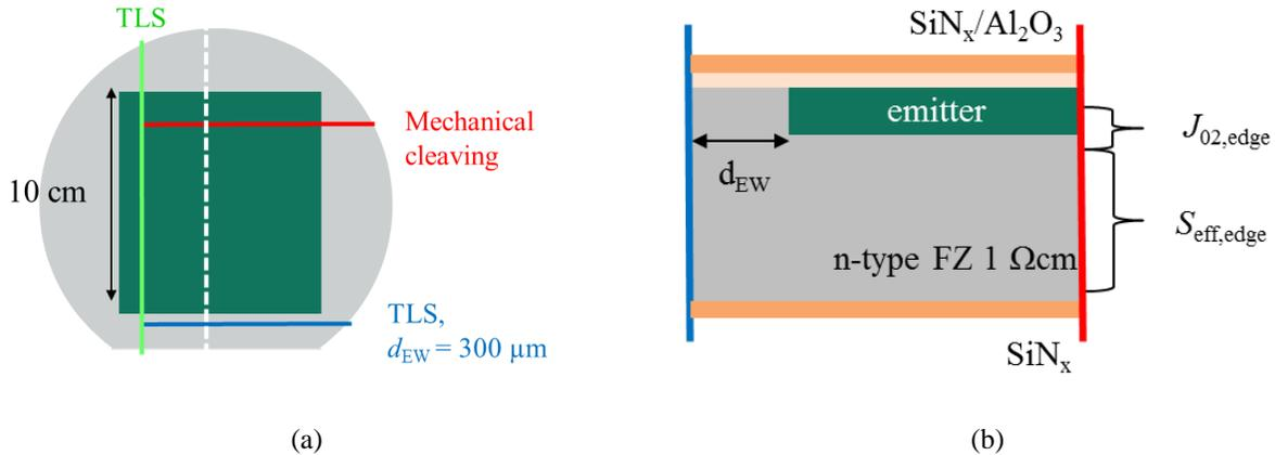
**FIGURE 1.** (a) Top-view sketch of the 6 inch wafers with emitter window (dark green) and indicated edge types (colored); (b) cross-section sketch (white dotted line in Fig. 1a) where the distance between emitter and edge is indicated by the parameter  $d_{\text{EW}}$ .
