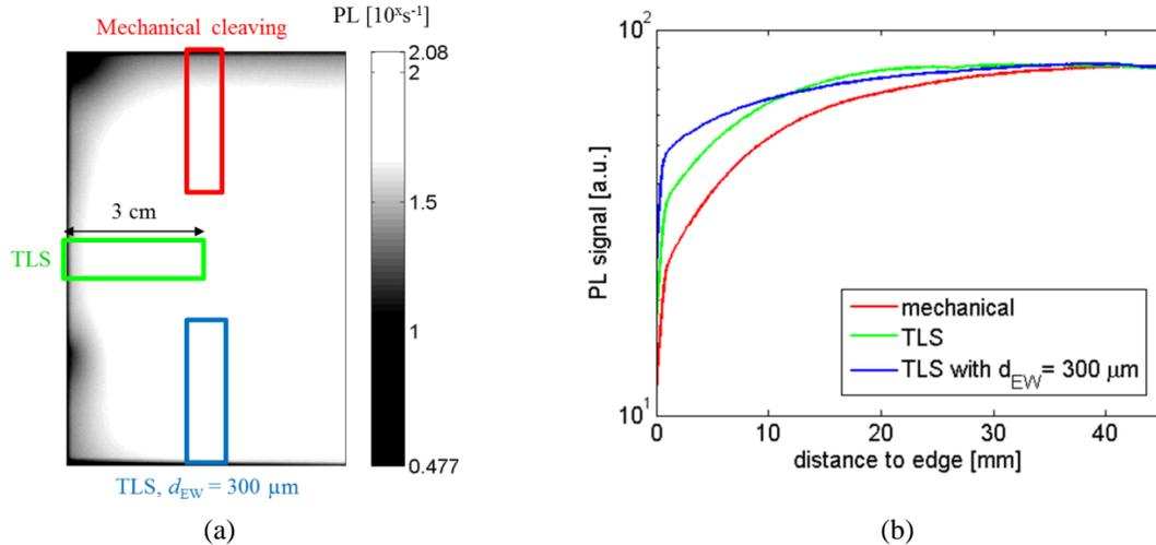
**FIGURE 3.** (a) Logarithmically scaled PL image at 0.02 suns shows the three differently affected edges and (b) the corresponding PL profiles averaged over the respective areas depicted by the rectangles.
