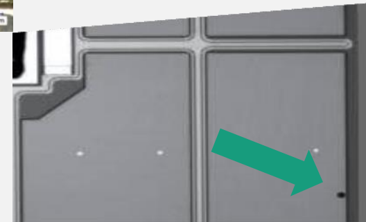
Localized defect on IGBT by lock-in thermography
