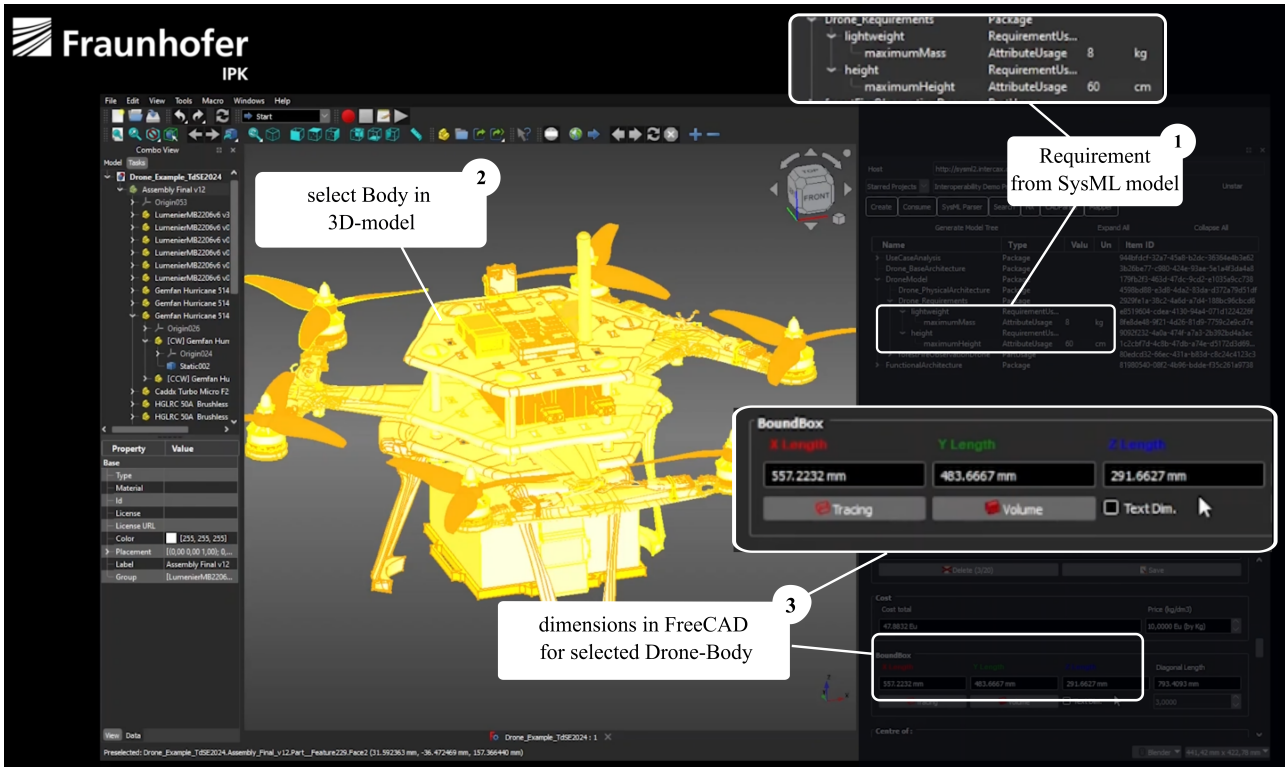
Figure 2: MCAD application FreeCAD with a dialog for interacting with the SysML v2 model on the IntercaX server via the API.
