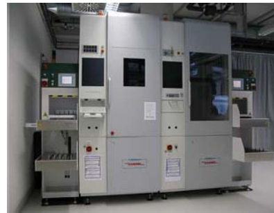
Figure 6: Photograph of the fully automated flash simulator for light and dark IV characterization of CPV receivers at Fraunhofer ISE.
