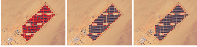
Fig. 2. Comparison of segmentation results at different resolutions for the Reggane PV system. From left to right: 20, 80, and 320 cm. The red overlay shows the results from segmentation.
