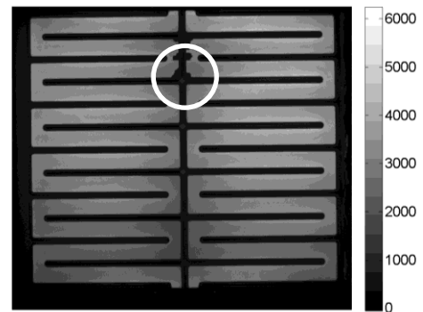
Figure 8: Two electroluminescence image of a 100 \text{ cm}^2 module measured at Fraunhofer ISE showing a mostly homogenous coloration. The circle indicates non-active areas due to in-sufficient electrolyte filling.
