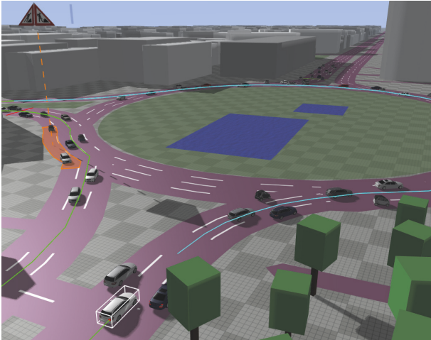
FIGURE 10: Simulator reference implementation, example scenario: construction site at round about, Ernst-Reuter-Platz, Berlin, Germany.
