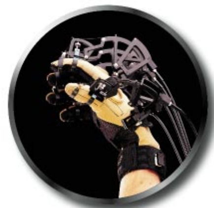
The mechanical force-feedback exoskeleton CyberGrasp by Virtual Technologies, Inc.
