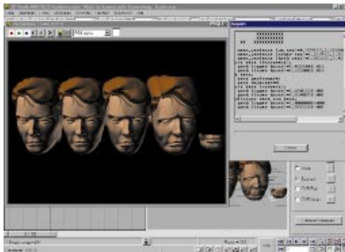
Retrieval of a robust watermark from complex transformed models (heads from left to right: original, watermarked copy, polygon simplification, free-form deformation, fragment)
