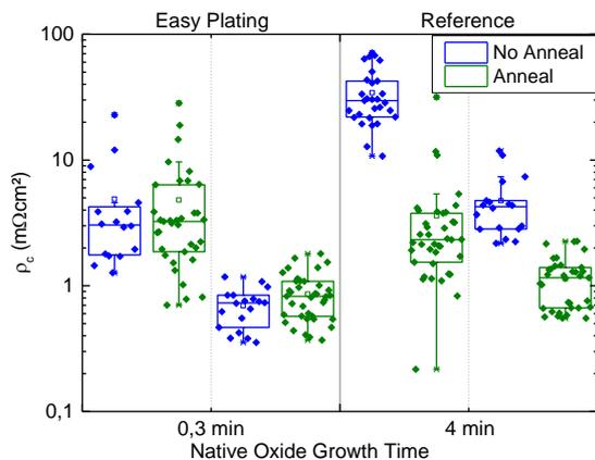
**Figure 5:** Results of contact resistivity at two different native oxide growth times between laser-ablation and HF-pre-treatment and laser-ablation and metal deposition for *Easy Plating* (left side) and *Reference* (right side), respectively. Process groups with and without anneal are colored green and blue, respectively.
