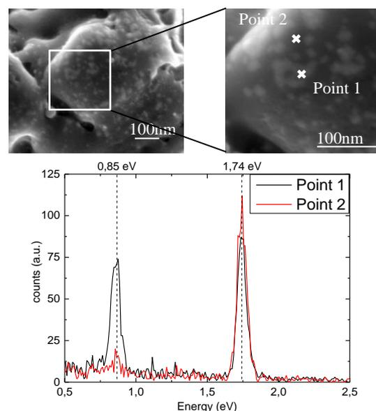
**Figure 7:** Top View SEM images of laser ablated surface after metal removal for *Reference* process with a native oxide growth time of 0.3 min (up). EDX measurement of two points in an area with and without silicide (down)
