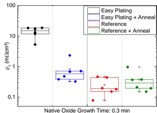
**Figure 9:** Contact resistivity for *Easy Plating* and *Reference* process before (black, red) and after (blue, green) anneal with a minimum native oxide growth time of 0.3 min
