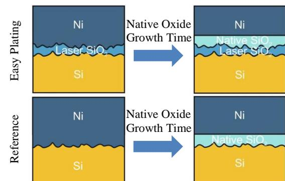
**Figure 4:** Schematic representation of the interface layers for the *Easy Plating* (up) and *Reference* (down) process and native oxide growth time between laser ablation respectively HF-pre-treatment (left) and plating (right).
