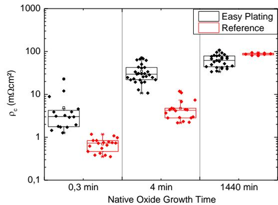
**Figure 3:** Results of contact resistivity for different native oxide growth times between laser-ablation respectively HF-pre-treatment and metal deposition for the *Easy Plating* (black) and *Reference* (red) process sequence.
