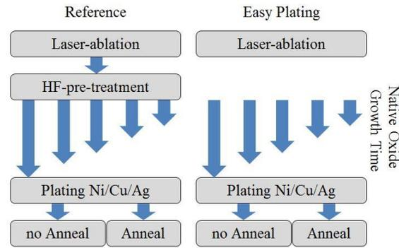
**Figure 2:** Process scheme of the experiment. Each process sequence features a variation of native oxide growth time before plating in which native oxides are grown at the contact interface
