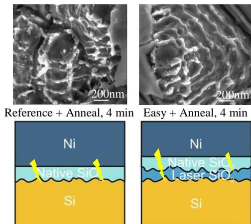
**Figure 8:** Top View SEM images of laser ablated surface after metal removal for *Reference* (up left) and *Easy Plating* (up right) process with a native oxide growth time of 4 min and the correspondent schematic layer structure (down) with local conductive channels
