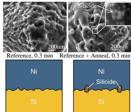
**Figure 6:** Top View SEM images and of laser ablated surface after metal removal for *Reference* process with a native oxide growth time of 0.3 min without (up left) and with anneal (up right) and the corresponding schematic layer structure before anneal (down left) and after anneal with local silicides (down right)
