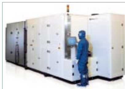
Lasermaskenbelichter von Micronic Laser Systems (SIGMA 7300) laser mask writer from Micronic Laser Systems (SIGMA 7300)
