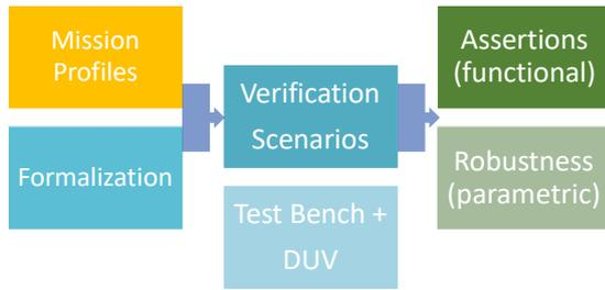
**Figure 2** Combination of mission profiles and formalized requirements for automated generation of verification scenarios
