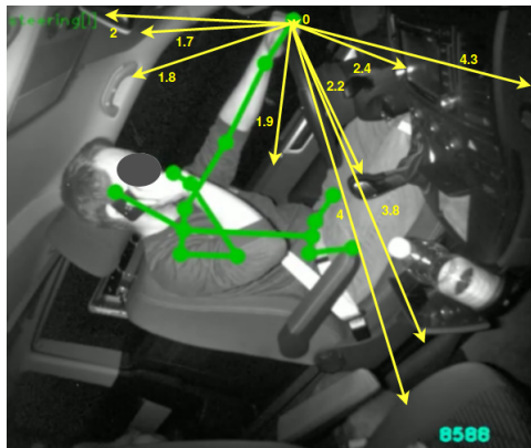
Fig. 3: Visualization of the context data represented as distances of the hands to different regions in the interior. The left hand grabs the steering wheel. The distance to the wheel is therefore zero. (best viewed in color)
