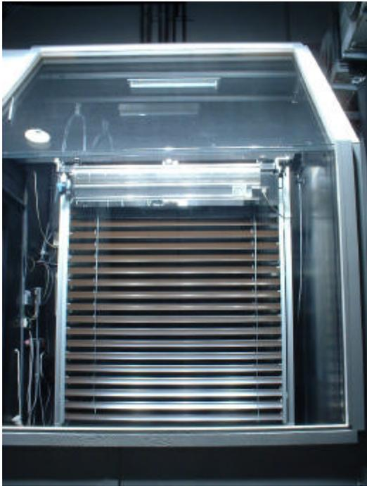
Figure 3: View into cabin on the Fraunhofer ISE solar calorimeter (measurement of a solar protection device)
