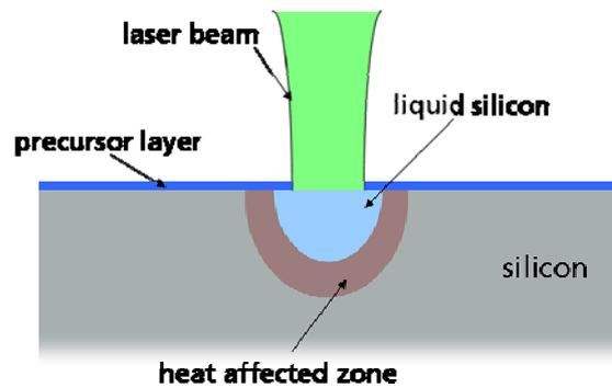
**Figure 1:** Principle of laser doping: a shallow region of the wafer is molten and a dopant is driven into the silicon during the liquid phase.
