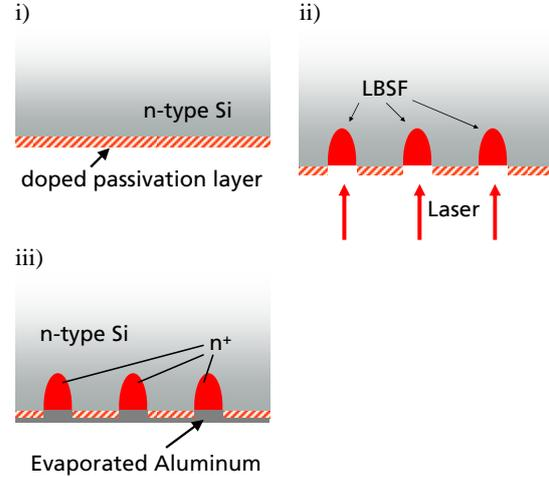
**Figure 3:** Process scheme of the *PassDop* approach: after cleaning, (i) a doped passivation layer is deposited onto the rear side of the wafer, (ii) a laser opens point contacts in the passivation layer and simultaneously dopes the substrate subsequently (iii) aluminum is evaporated on top finishing the rear side of the device [15].
