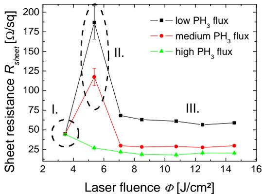
**Figure 4:** Evolution of the sheet resistance with increasing laser fluence  $\phi$ . After crossing the melting threshold, the sheet resistance changes only little for a given precursor layer. The three different  $\text{PH}_3$  gas fluxes are shown. The three regions are explained in the text.
