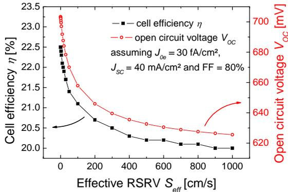
**Figure 2:** Dependence of the open circuit voltage  $V_{\text{OC}}$  and cell efficiency  $\eta$  on the effective rear side recombination velocity for a high efficiency  $n$ -type PERL solar cell
