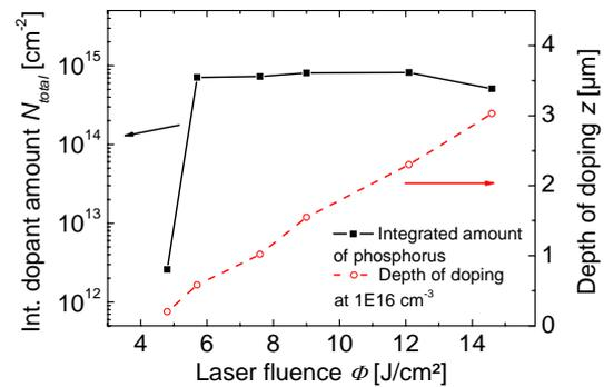
**Figure 6:** Integrated amount of phosphorous after laser doping and depth of doping at  $1e16 \text{ cm}^{-3}$  [15].
