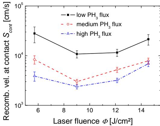
**Figure 7:** Recombination velocity at the contact  $S_{cont}$  as a dependence of the laser fluence  $\Phi$  and with the gas flux as a parameter [15].
