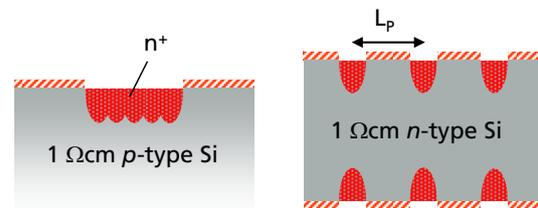
**Figure 4:** Left: Samples prepared for the investigation of the doping (i) and Right: samples prepared for testing the local point contacts (ii)
