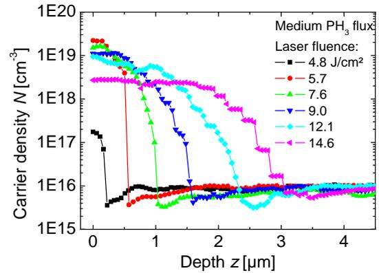
**Figure 5:** Resulting doping profiles after laser irradiation. The profiles displayed are for the medium flux of  $\text{PH}_3$  [15].
