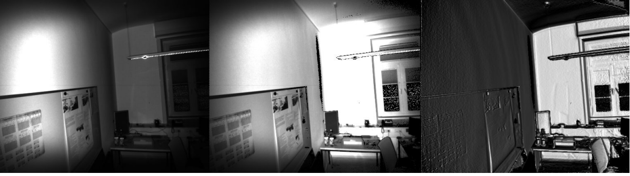
Figure 5. Planar wall recorded for the plane fitting test. The images are an IR intensity image truncated to 8 bit showing the illumination falloff with increasing distance, illumination normalized by distance and a visualization of the estimate surface normal of every pixel. The intensity is defined as the euclidean norm of two corresponding correlation coefficients.
