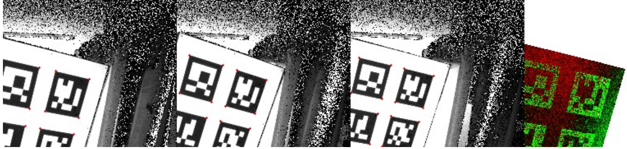
Figure 3. Reflections of the whiteboard influence measurements on the marker board and vice versa. The noise on the whiteboard moves according to the position of the marker board as can be seen in the first three images. The relative distance error has been visualized in the last image. Overestimated distances are shown in green, underestimated distances in red. Dark parts of the board show a intensity related depth bias.
