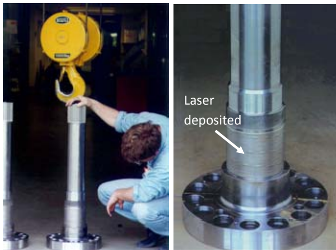
Figure 15: Repair of centrifuge axis [21]
