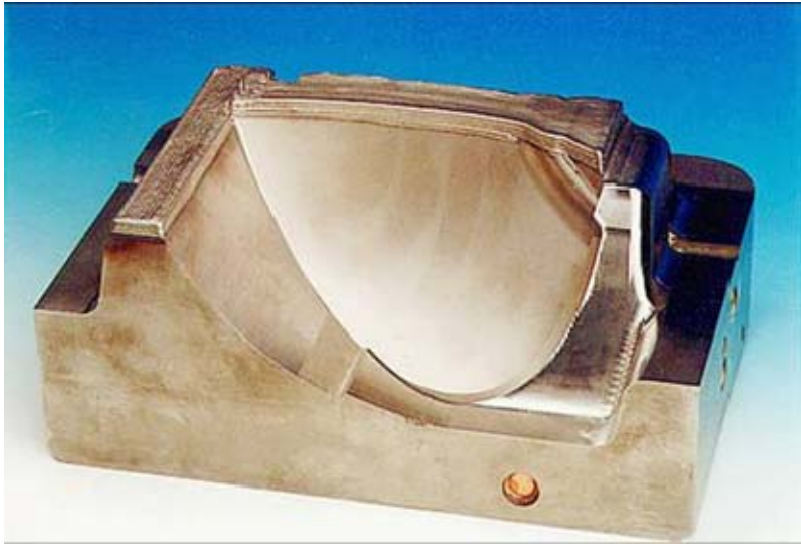
Figure 13: Modification of an injection mould for a car lamp housing (material: hot working steel) [24]
