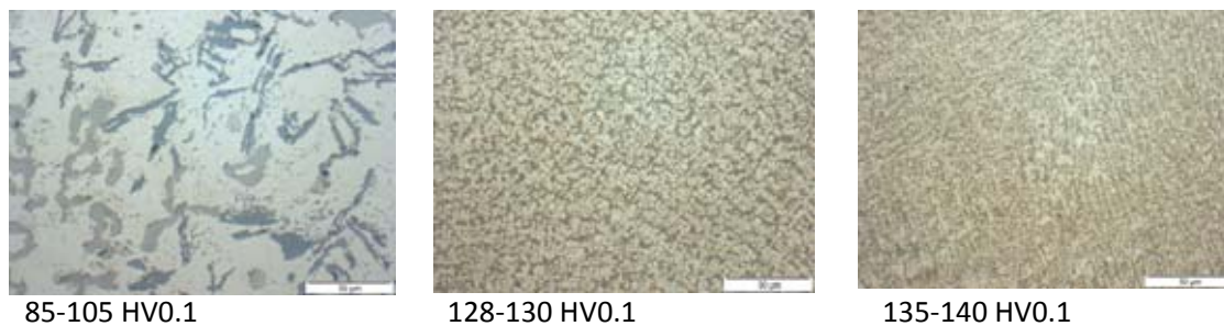
Figure 3: Grain refinement in the alloy AlSi10Mg after laser remelting [16], P = 1 \text{ kW} , d_L = 1 \text{ mm} ; left: substrate, centre: v_v = 0.5 \text{ m/min} , right: v_v = 5 \text{ m/min}
