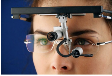
Figure 2: Head unit of the eye tracker system [8]
