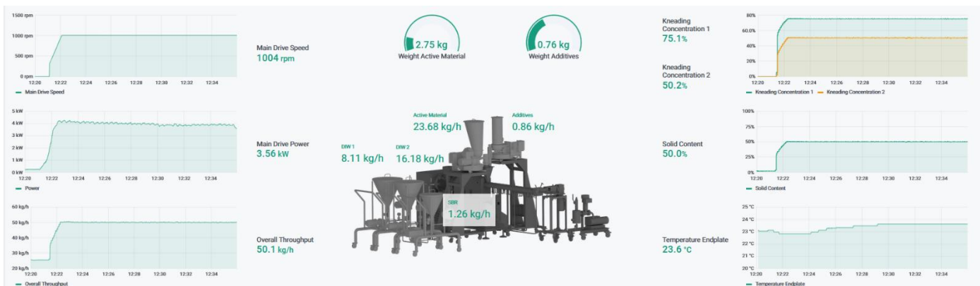
Fig. 4. A dashboard for the extrusion experts allowing them to gain insight to the process parameters of the digital machine twin.
