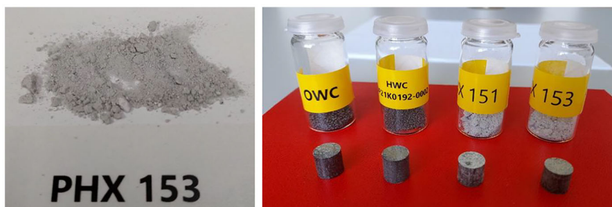
FIGURE 3 | Granulate of the cocrystal formulations PBX-formulation of the FhG ICT (PHX) 153 (left) and granulate samples and pressed pellets used for the microstructure characterization (right).
