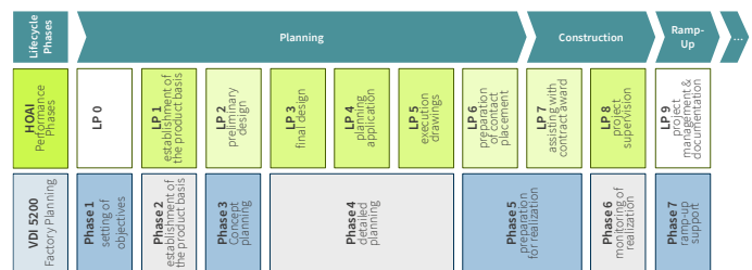
Fig.2: Assignment of the HOIA and the VDI 5200 Phases (own representation based on [15])
