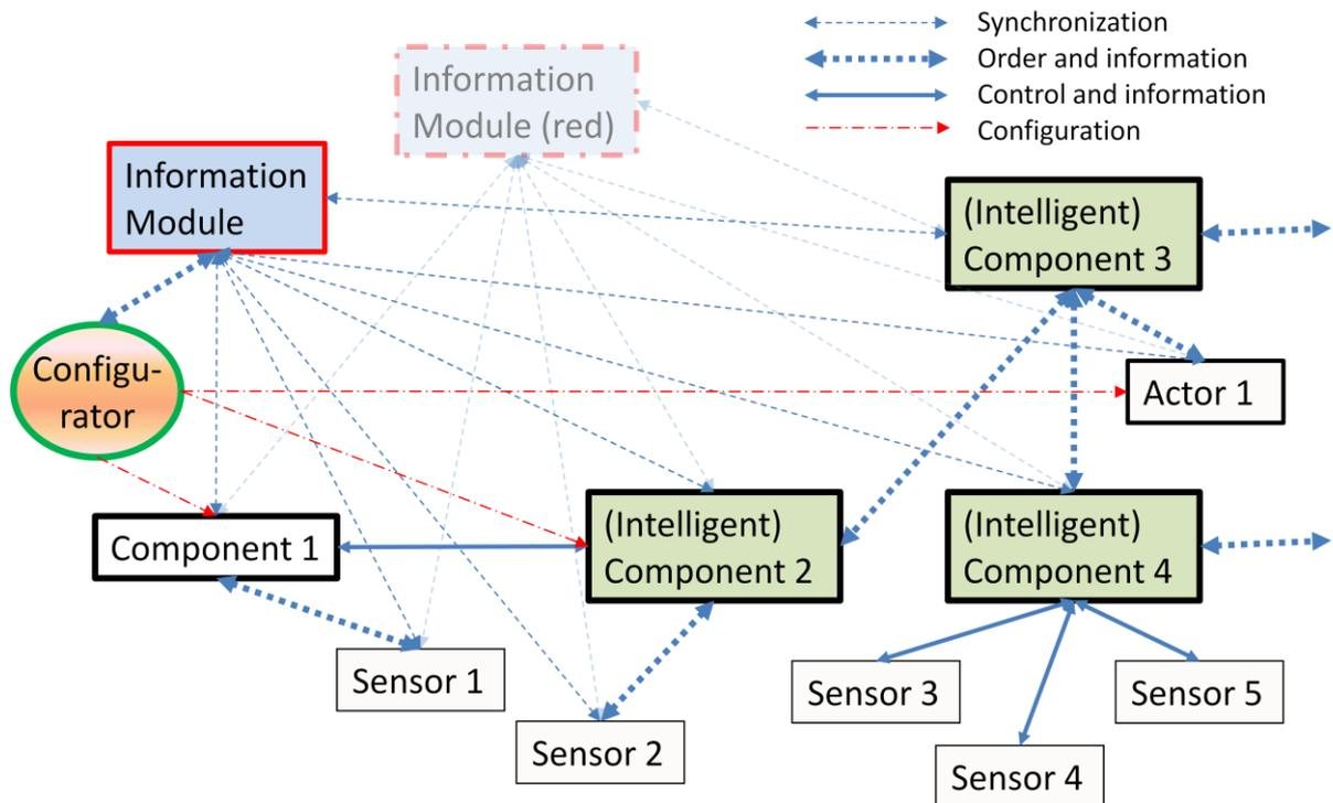
Fig. 1: A sample structure of automatically configurable distributed system with heterogenic components
