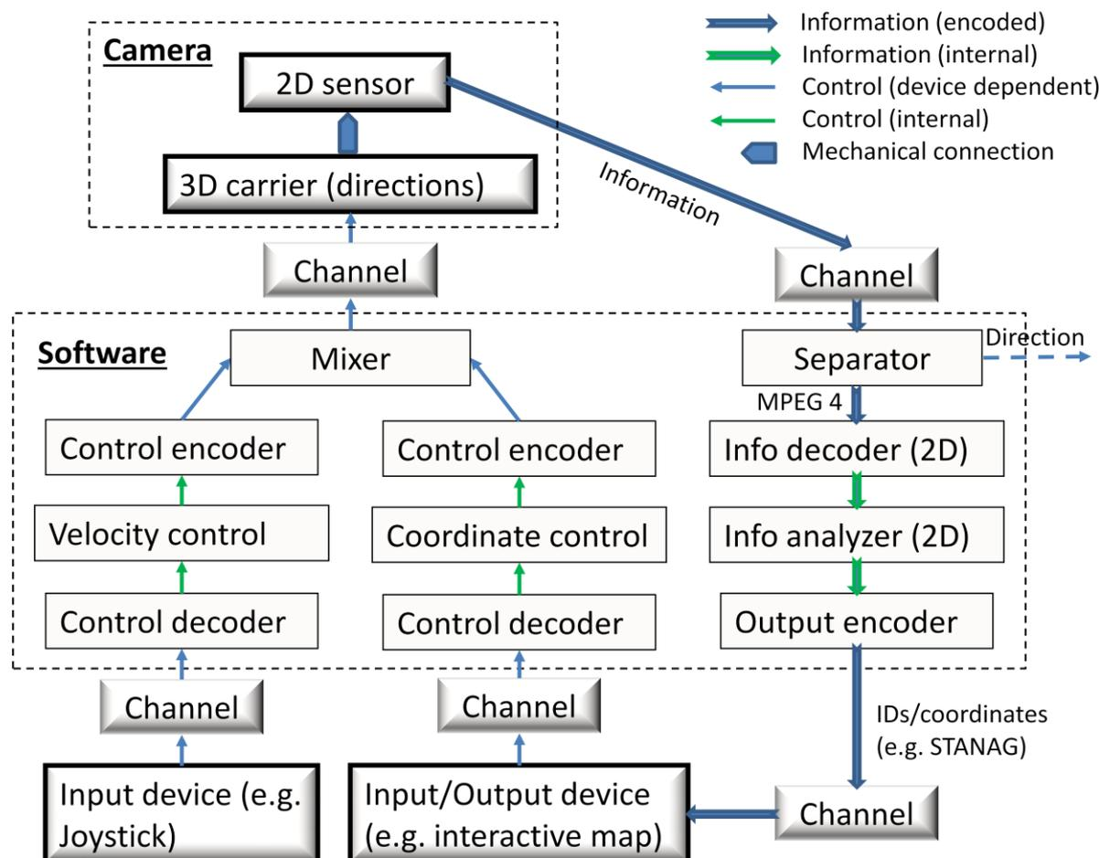
Fig. 7: Automatic configurable information analyzing and control system for pan-tilt camera
