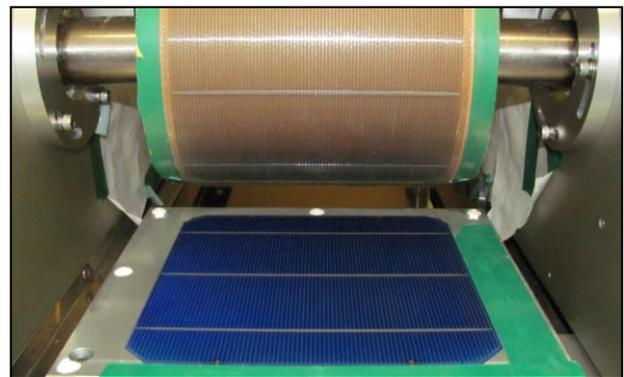
**Fig. 1** Experimental platform for solar cell metallization using flexographic printing
