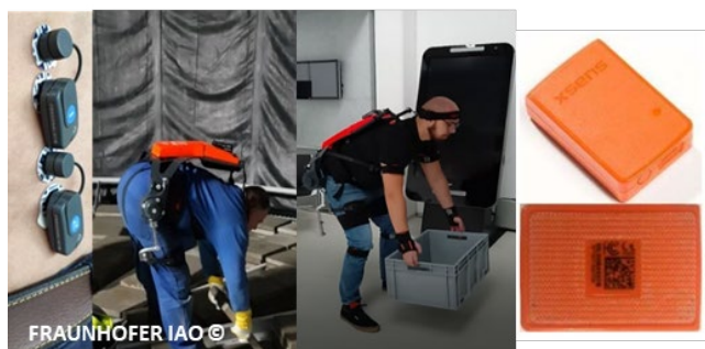
Fig. 2. Electromyographic study of the lower back - Erector spine at the workplace level (left), Motion capture using Xsens technology (right)
