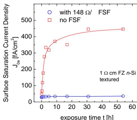
**Figure 3.** Passivation stability of textured  $n^+nn^+$  lifetime samples with and without FSF during 55 hours of exposure to UV-light. Lines are guides-to-the-eye.
