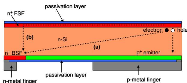
**Figure 4.** Schematic drawing of the effect of the enhanced lateral current transport of the majority carriers via the front surface field (symmetry element of the cell is shown). For simplicity the front side texture is not shown. The lateral current transport through the FSF (b) can be seen as an additional transport path to the base lateral resistance (a).
