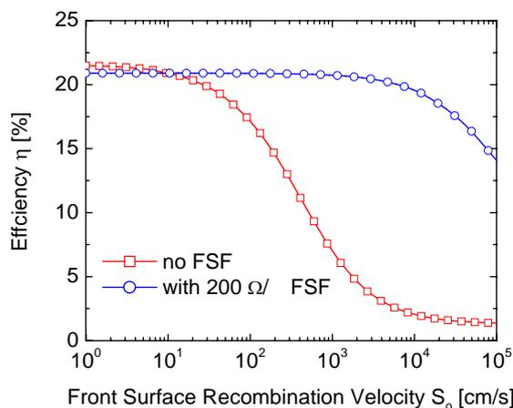
**Figure 2.** Influence of the front surface recombination velocity ( $S_{0,front}$ ) on the efficiency of back-junction  $n$ -type Si solar cells with and without the FSF (one-dimensional PC1D [5] simulations).
