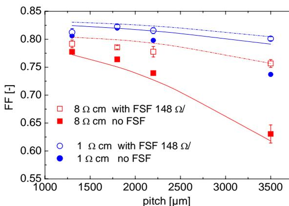
**Figure 5.** Fill factor of the processed cells and two-dimensional numerical simulations as a function of the pitch for two different base resistivities. Results for the cells with ( $\rho_{\text{sheet}} = 148 \Omega/\text{sq}$ ) and without FSF diffusion are shown. The data points represent a mean value of the experimental results. Lines represent the 2D simulation results.
