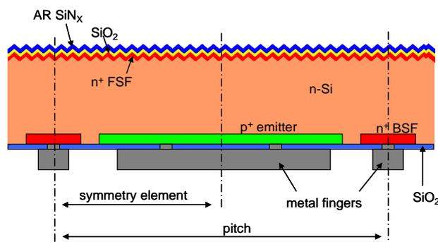
**Figure 1.** Schematic cross-section of the *n*-type high-efficiency back-contact back-junction silicon solar cell processed at Fraunhofer ISE (sketch is not to scale). Pitch and the symmetry element used for two-dimensional device simulations are shown.
