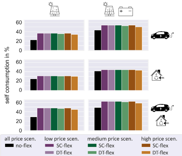
Fig. 6. Average self-consumption rate for the SC-flex and DT-flex case for all three price scenarios.
