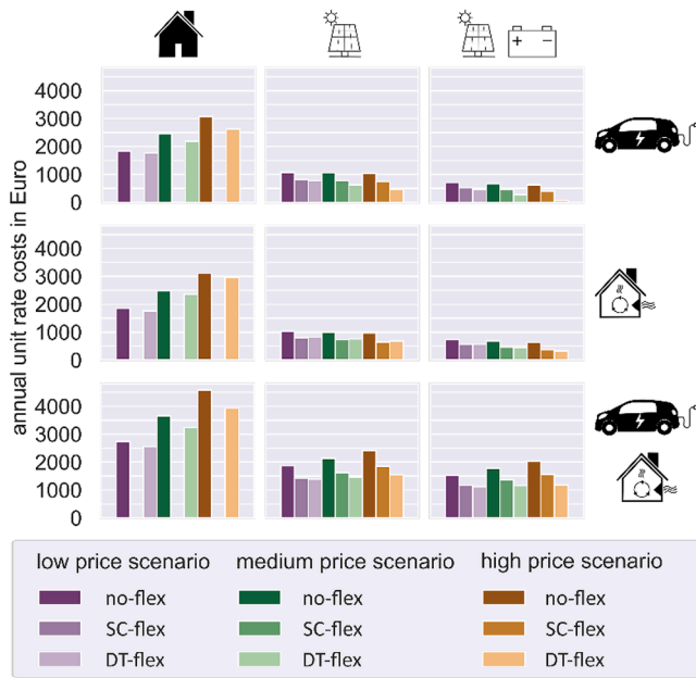
Fig. 7. Annual unit rate costs for the no-flex, SC-flex, and DT-flex cases for all three price scenarios (average over all households).
