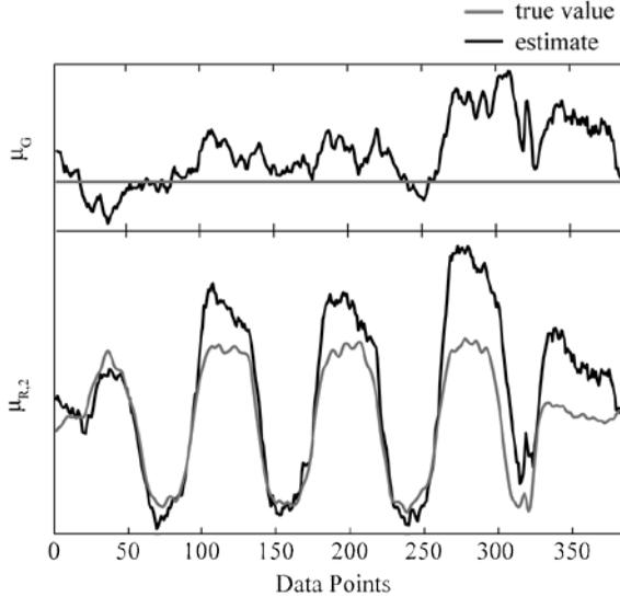
**Figure 5** – In this example, estimation of  $\mu_G$  (black line, above) gets worse between time step 250 and 370. Accordingly, estimation of  $\mu_{R,2}$  (black line) deviates from the true values for  $\mu_{R,2}$  (grey line) too
