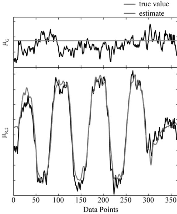
**Figure 4** – Example of good estimation of  $\mu_G$  (black line, above) that also leads to good estimation of  $\mu_{R,1}$  (black line). The true values for  $\mu_G$  and  $\mu_{R,1}$  are plotted grey lines, respectively.
