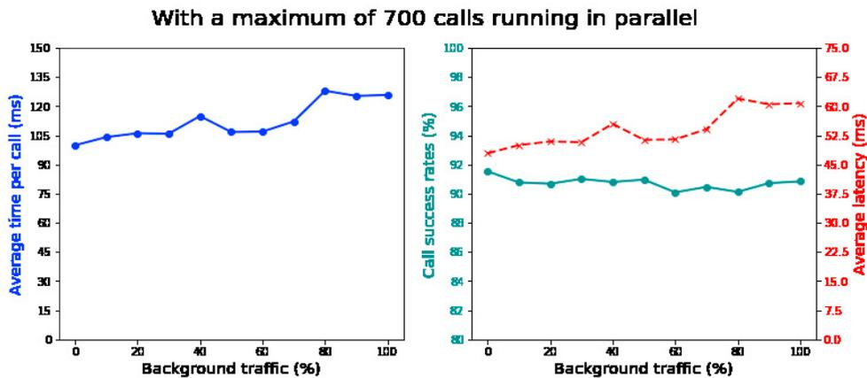
Fig. 5: SIP Call Establishment with a maximum of 700 calls in parallel
