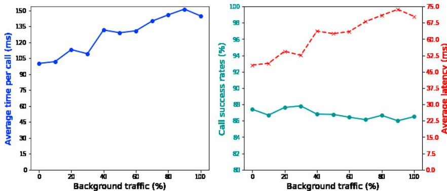
Fig. 6: SIP Call Establishment with a maximum of 1000 calls in parallel
