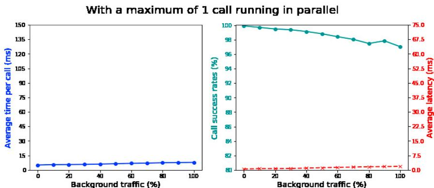
Fig. 3: SIP Call Establishment with maximum 1 call in parallel
