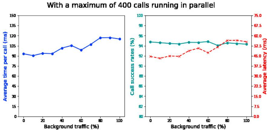
Fig. 4: SIP Call Establishment with a maximum 400 calls in parallel
