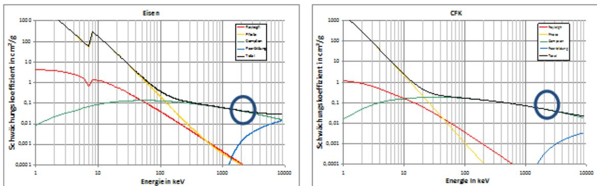
Figure 3: Absorption mechanisms dependent on X-ray energy for different materials. Left: Iron (Fe), Right: CFRP. The marked position represents the average energy of the high energy X-ray spectrum produced by 9 MeV SILAC source.
