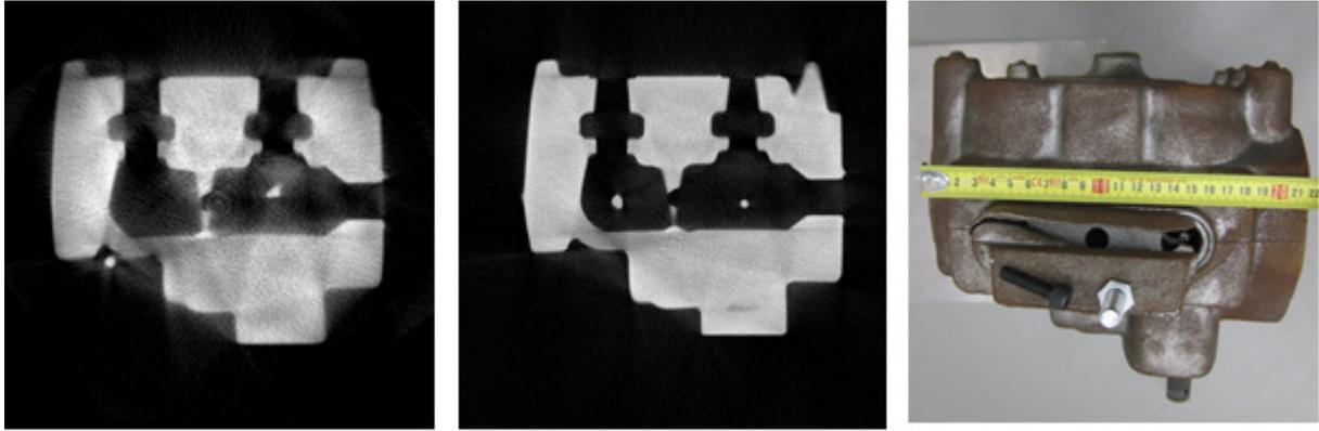
Figure 5: Comparison of a cone beam scan using a Flat Panel Detector (left) and a fan beam scan using a linear detector array (center) at 9 MeV. Photograph of the original iron casting part (right).
