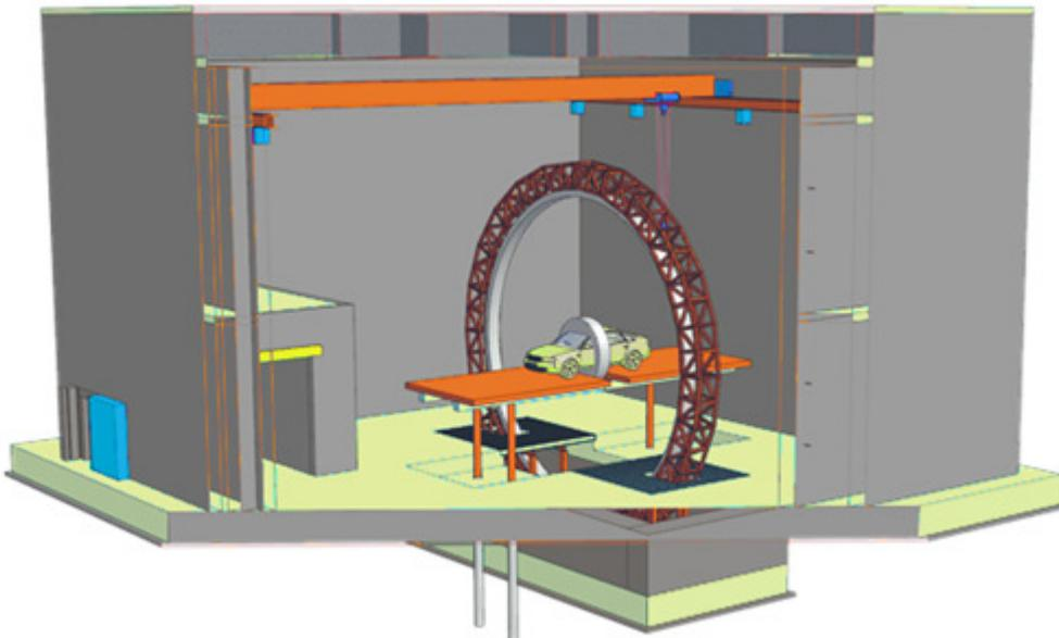
**Figure 7: 3D drawing of the final development stage planned for the CT-scan of long objects in their native orientation.**
