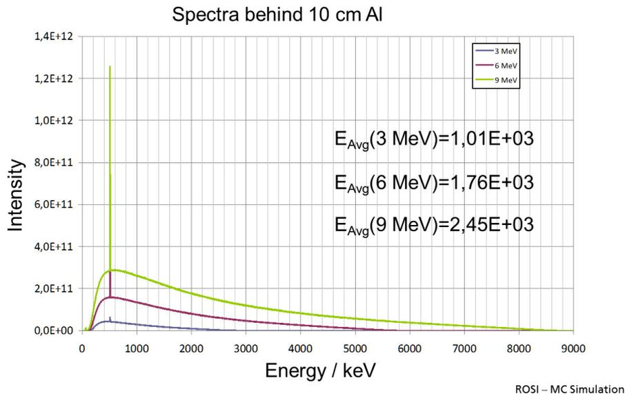
Figure 2: High-Energy X-ray spectra at 3, 6 and 9 MVp. The average energy remains in the region between 1 and 2.4 MeV.
