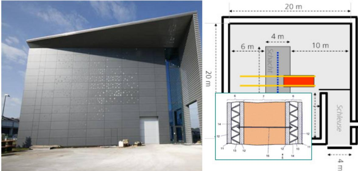
Figure 1: High Energy X-ray facility (left). Schematic drawing of the X-ray chamber with double layered walls and dimensions (right).
