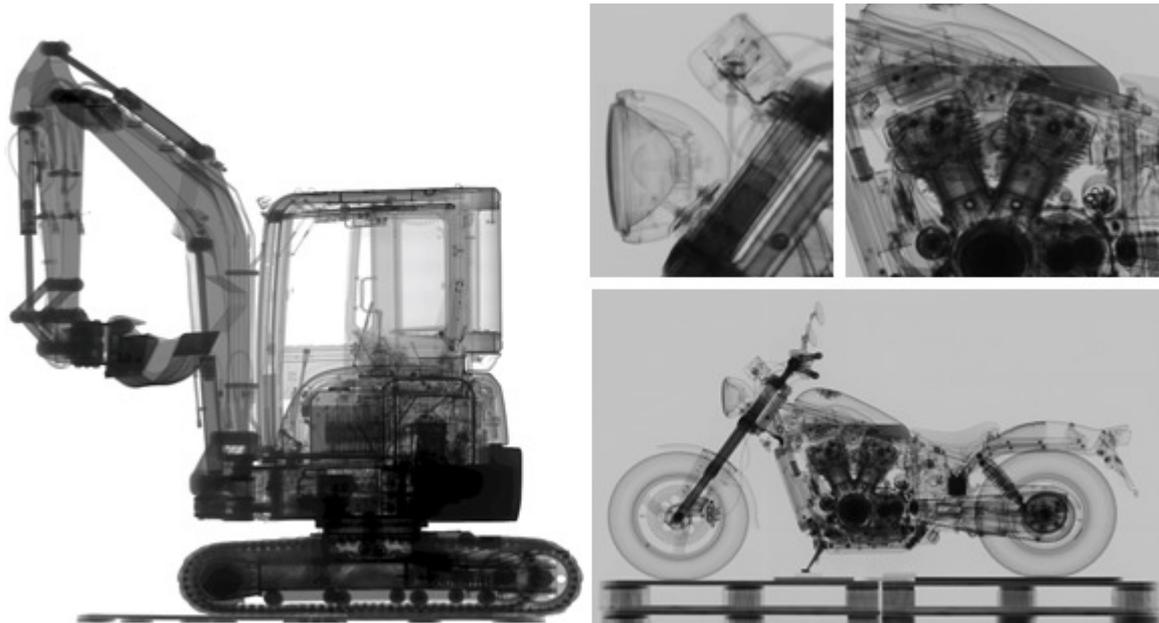
Figure 8: Radioscopy of large machines. Digger with approx. 3 t weight (left), Motorcycle with low fuel (right). Even in the regions of high absorbing materials details of the interior are recognizable.
