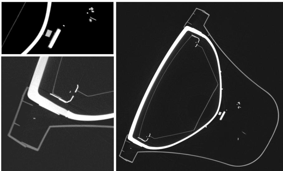
Figure 9: Cross-section of a television tube scanned with 9 MeV. The tube made of lead-glass gives a good contrast to the remaining materials in the TV. Differently than with lower energy scans, image quality is not affected by the high-absorbing material.
