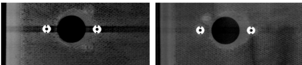
Figure 4: Comparison of a low energy scan at 450 keV(left) to a high energy scan at 9 MeV(right). The iron inlays caused metal artifacts due to the predominant photo effect with radiation of 450 keV. These artifacts do not occur in the high energy scan.
