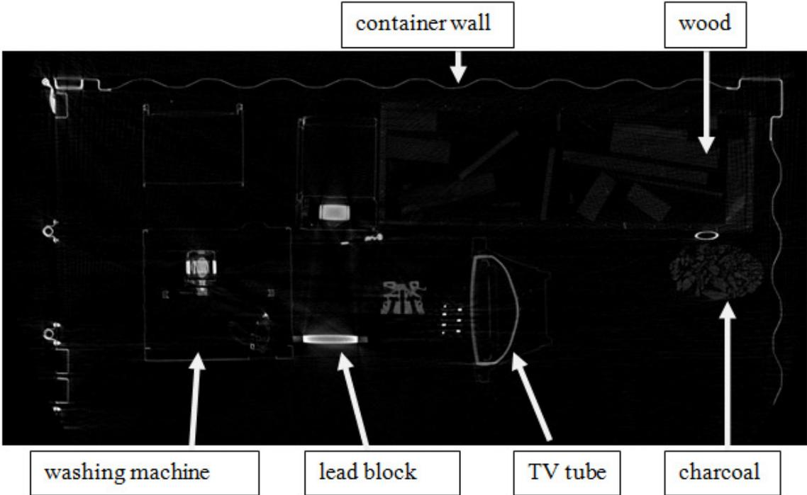
**Figure 10: Feldkamp reconstructed cross section of a loaded 20 ft sea-fright cargo container with differently absorbing materials.**
