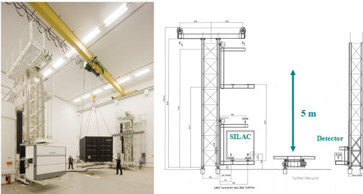
Figure 6: Photograph of the realized scanner Stage 1 (left). Drawing of the stage 1 setup with the SILAC (3 t) and the detector (1 t) providing a scan area of  $3.2 \times 5\ \text{m}$  (right).
