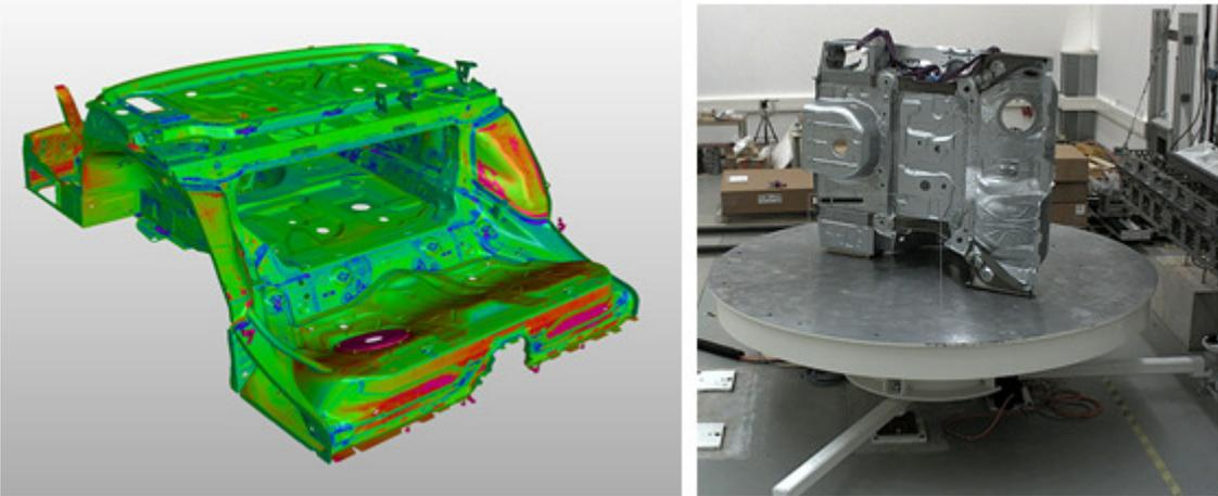
**Figure 11: Body rear end of a car. The image quality of the scan allows for a metrological analysis, such as a variance analysis (left). A photograph of the object can be seen on the right.**
