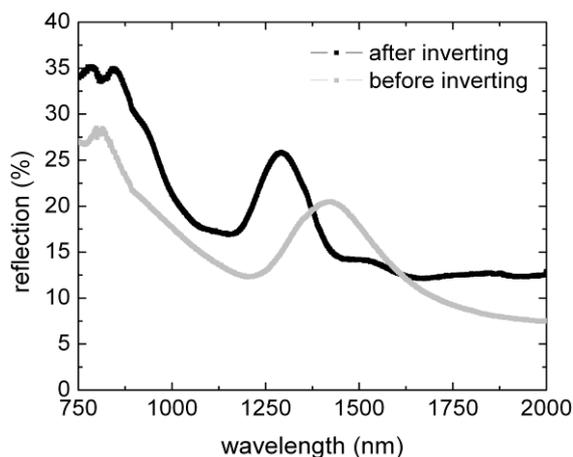
**Figure 6:** Reflectance measurements of the  $\text{Si}_y\text{C}_{1-y}$  photonic structure (light grey) and after (black) burning out (inverting) of the PMMA spheres.
