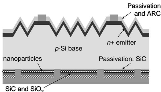
**Figure 1:** Sketch of the high efficiency solar cell structure with photonic crystals (PC) on the rear side.
