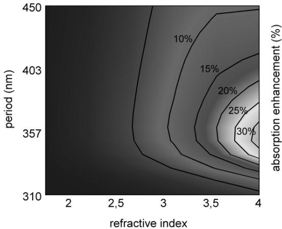
**Figure 2:** Dependency of the relative absorption enhancement on the photonic crystal period and its refractive index for a silicon solar cell without front side texture.
