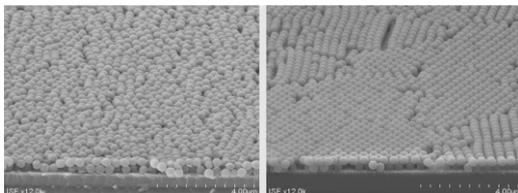
**Figure 3:** Scanning electron micrograph (SEM) of PMMA nano spheres spin coated on  $\text{Si}_x\text{C}_{1-x}$  (left) with an over diluted solution and (right) with optimal dilution and spin coating parameters.
