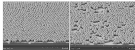
**Figure 4:** SEM of a monolayer of  $\text{SiO}_2$  nano spheres deposited on  $\text{Si}_x\text{C}_{1-x}$ .
