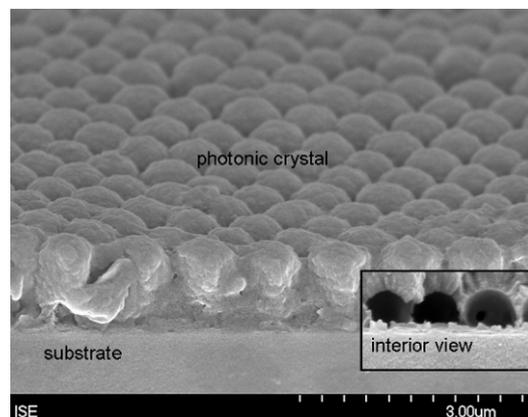
**Figure 5:** SEM of the  $\text{Si}_y\text{C}_{1-y}$  photonic crystal structure on a glass substrate.
