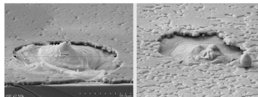
**Figure 7:** SEM pictures showing the back side contact opening with laser ablation, with a power of 5.45 W and 1 repetition (left) and a power reduced to 3.75 W and 3 times lasering on each contact (right).
