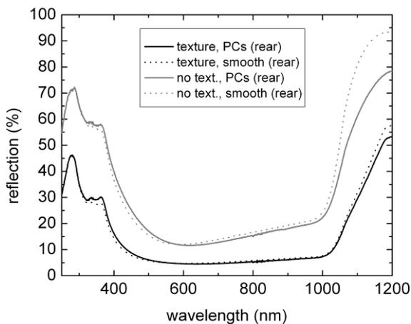
**Figure 8:** Reflection measurement over wavelength for different solar cell structures with textured front side (black) and/or photonic crystals on the rear side (solid).
