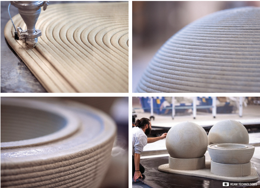
Figure 6: Photographs of 3D Stored Energy in the Sea (StEnSea) proof-of-concept print by RCAM Technologies and Vertico.
