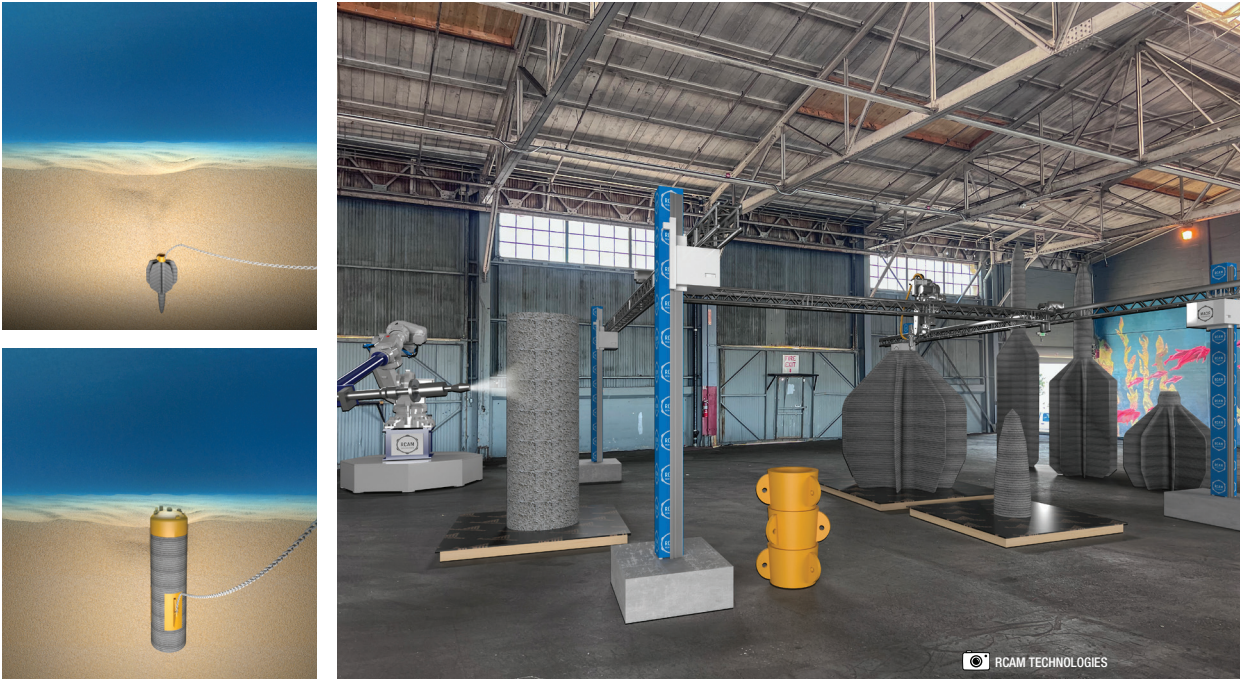
Figure 5: Artist's renderings of 3D concrete printed torpedo and suction anchor technologies for floating offshore wind.
