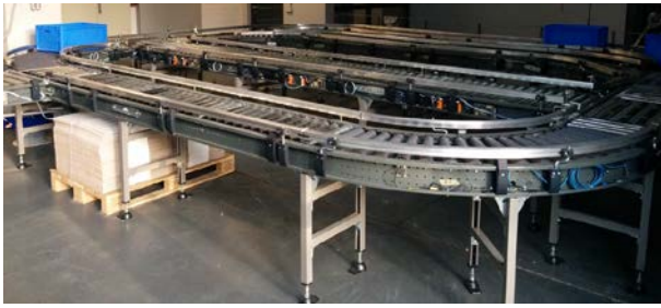
Figure 2. Example of plant consisting of Gebhardt conveyor modules
