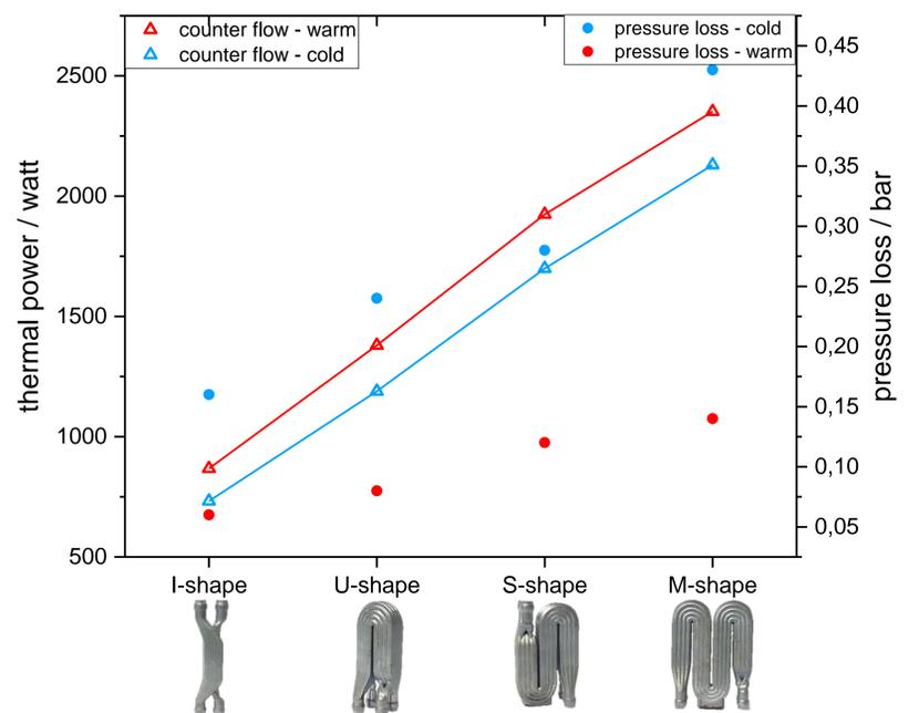
Fig. 4: Summary of results, showing the thermal power and pressure loss, depending on the geometry (I-, U-, S- and M-shape)
