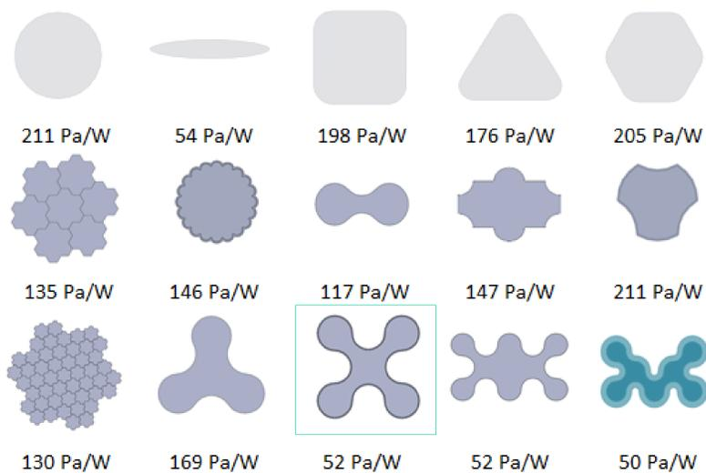
Fig. 1.: Summary of the investigated profile geometries, showing the pressure loss per thermal power
