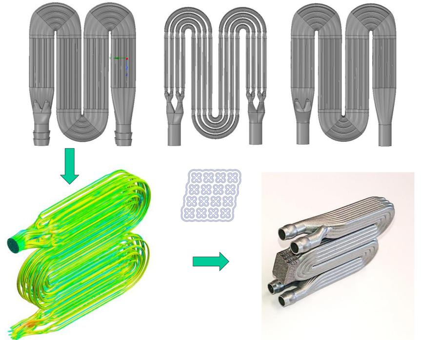
Fig. 3: Development process of additively manufactured miniature heat exchangers
