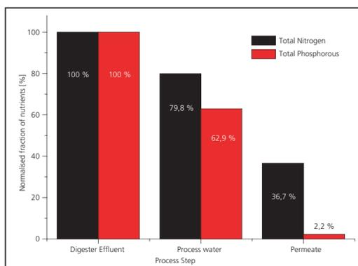
Figure 2: Concentration of nutrients after dewatering and Cross-Flow filtration with HITK e.V. 200 nm, tubular membrane ( $\alpha$ -Al<sub>2</sub>O<sub>3</sub> ceramic)
