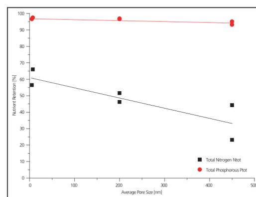
Figure 3: Retention of Nutrients as function of pore size of different membrane types
