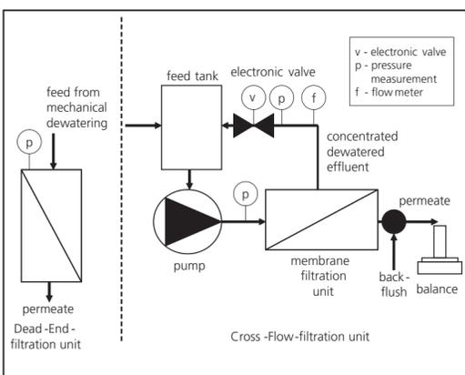
Figure 1: Schematics of lab-scale micro filtration membrane units (left: Dead-End-filtration unit; right: Cross-Flow filtration unit)
