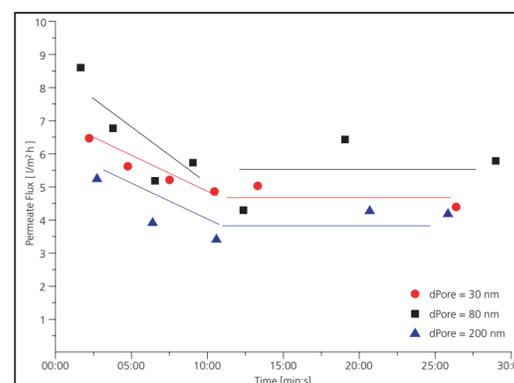
Figure 4: Permeate flux as function of process time for different flat Cross-flow membranes (Microdyn Nadir membranes; pore sizes: 30, 80, 200 nm; materials: PES, PVDF, PVDF)
