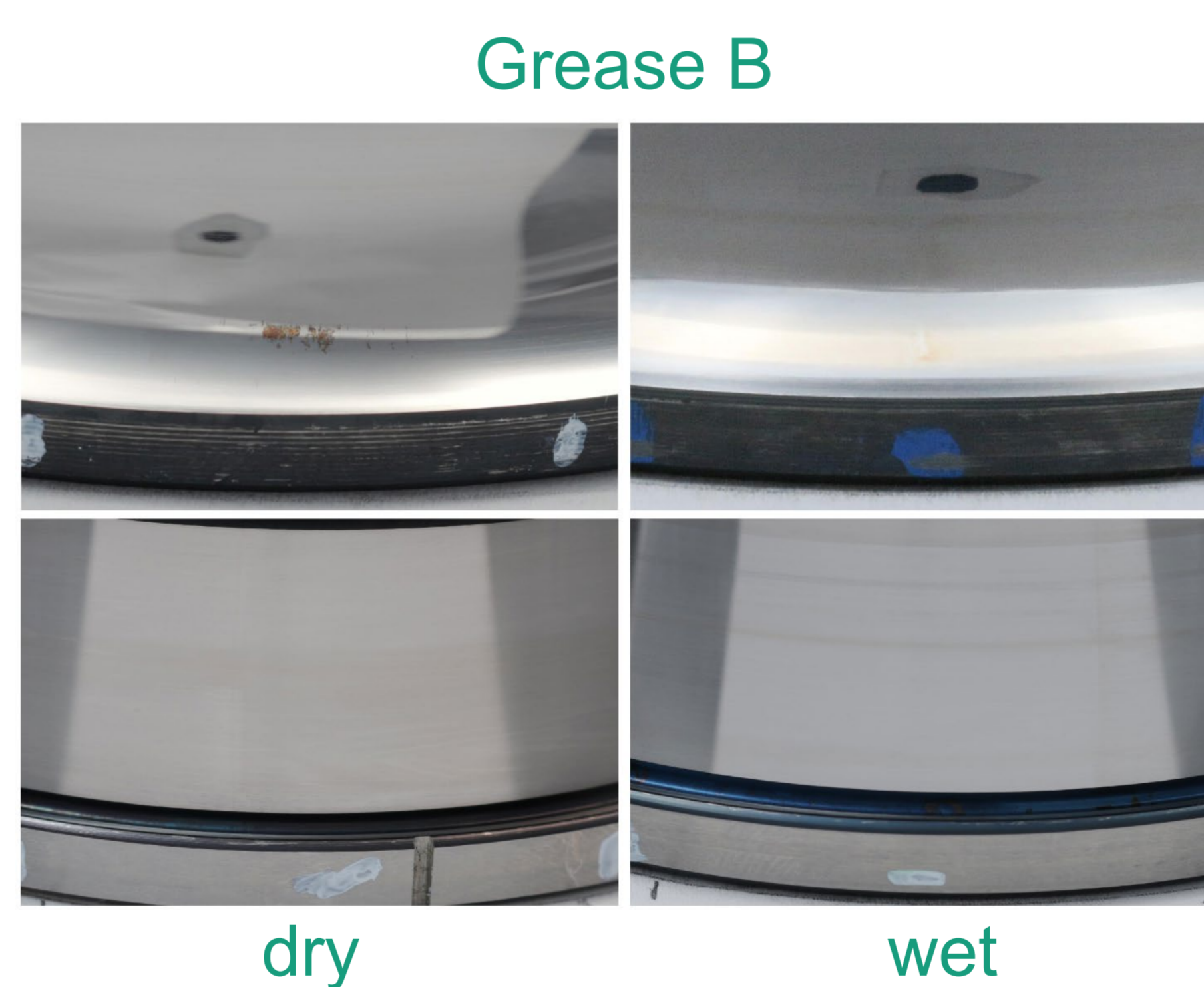
Figure 5: Raceway condition grease B after test
