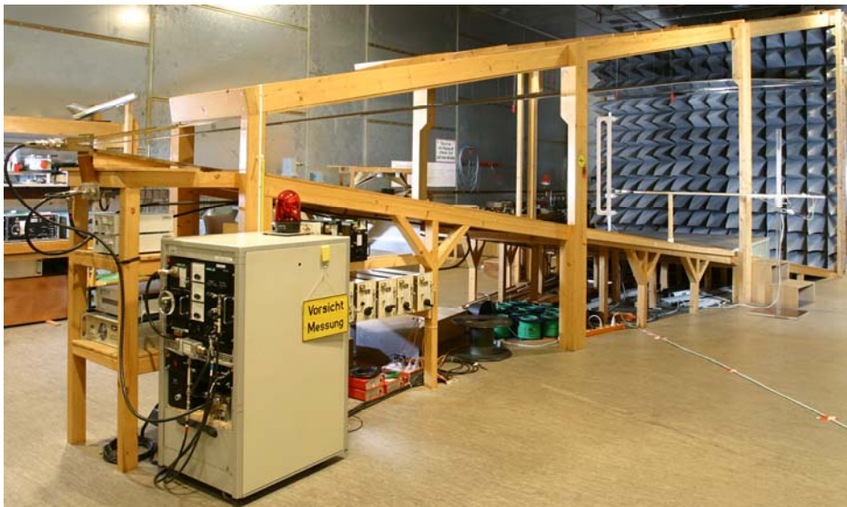
Figure 2: Photo of INT waveguide with pulse generator and DUT.
