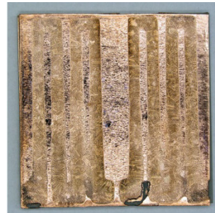
Fig. 2. Destroyed copper metallisation after active metal brazing of copper to AlN with the Ag-Ti braze.
