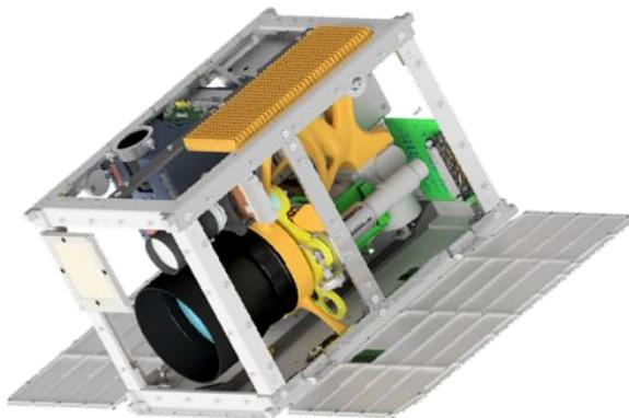
Fig. 2: CAD-Model of the ERNST satellite. The 3D-printed parts are highlighted with orange color.
