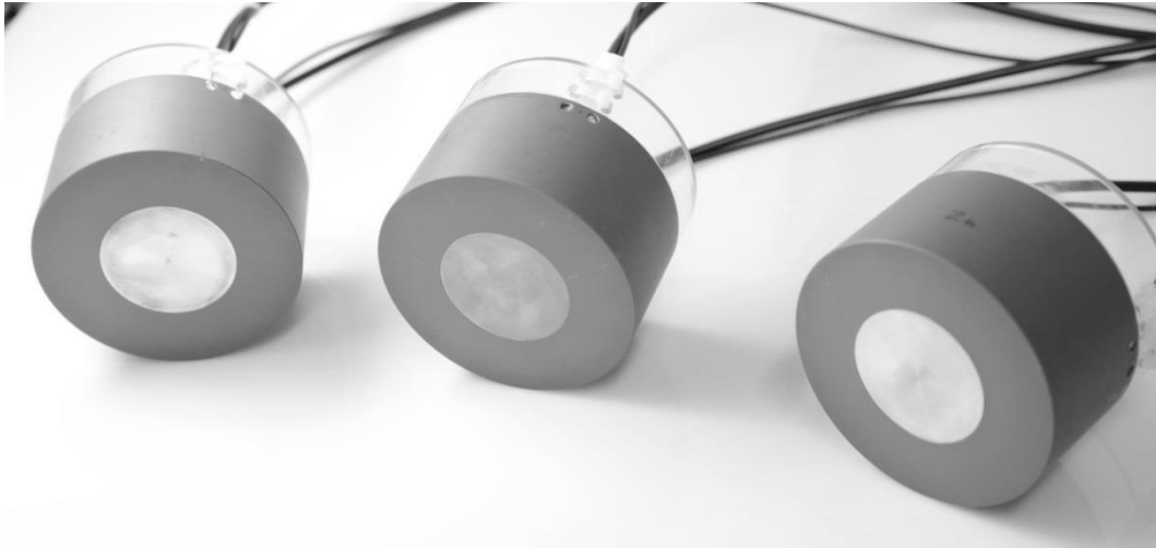
Figure 3: Ready to use targets with manganin gauges embedded in three different target materials
