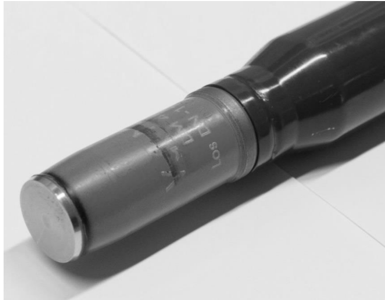
Figure 1: Modified projectile tip with 2 mm copper plating
