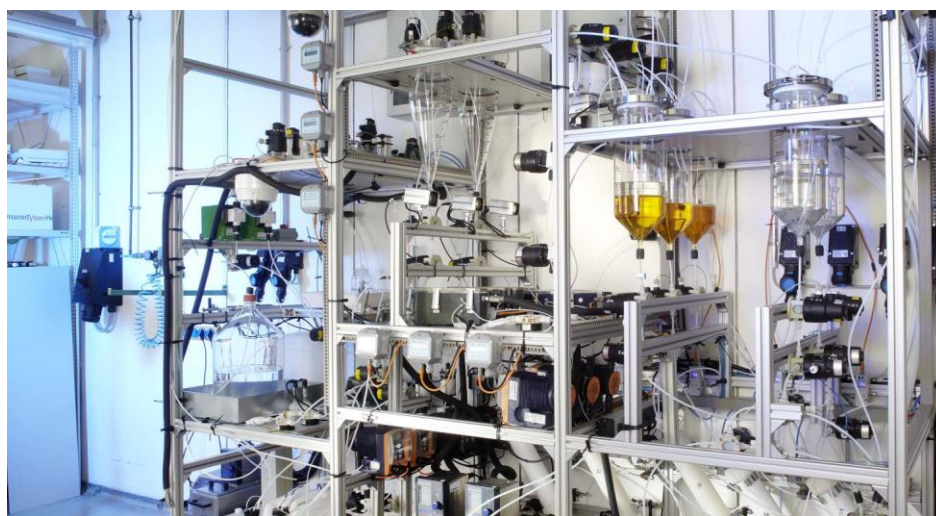
Fig. 3: Plant for continuous kg-scale synthesis of nitrate esters
