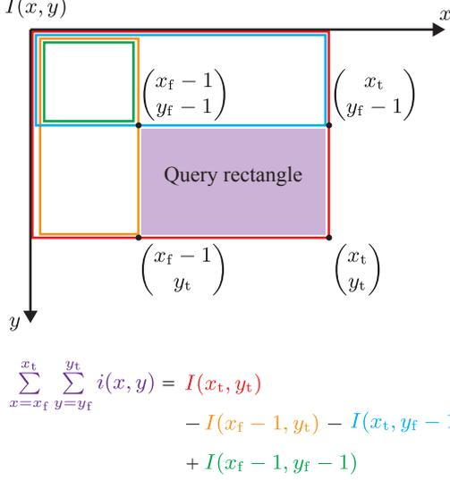
Figure 1: Calculating the sum of the array entries inside the query rectangle  $x \in [x_f, x_t]$ ,  $y \in [y_f, y_t]$  (purple) by employing a summed area table: from the red component  $I(x_t, y_t)$ , first the orange component  $I(x_f - 1, y_t)$  and the blue component  $I(x_t, y_f - 1)$  have to be subtracted. Since the area represented by the green component has now been subtracted twice,  $I(x_f - 1, y_f - 1)$  has to be added.
