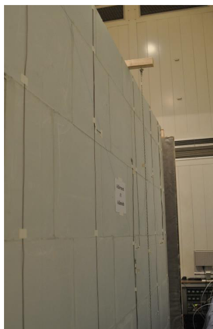
Fig. 2. Room in room system in the climate chamber. One outer wall of the test room in the climate chamber
