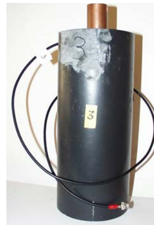
Figure 2. Armature X-Ray (Copper 40x2x300 mm, Composition B 523 g).
