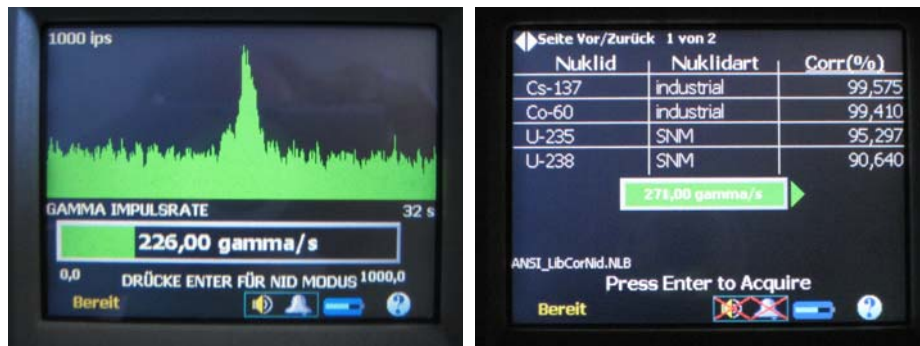
Figure 3: Left : Search mode, gamma counting rate versus time. The displayed peak represents a source which was passed during the searching process. Right : Identification mode with name of found nuclide, kind of nuclide and correlation to database. The example shows a measurement with ^{137}\text{Cs} , ^{60}\text{Co} and depleted uranium.
