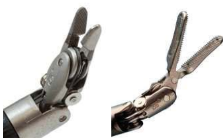
Figure 2.8: EndoWrist Needle holder on the left and grasper on the right
